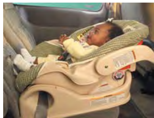
This car seat is installed correctly. It is at a 45° angle.
