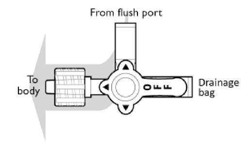
7. Turn the switch so it points to the flush port again (see drawing below). The word "OFF" (which is on the longest part of the stopcock) will be closest to the flush port. Your drain will now drain into the bag.
